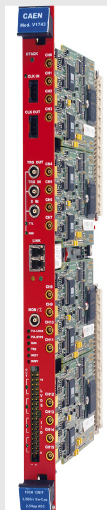
Fig 2: A photo of the CAEN V1743 digitizer used in developing pulse shape discrimination techniques [2]
